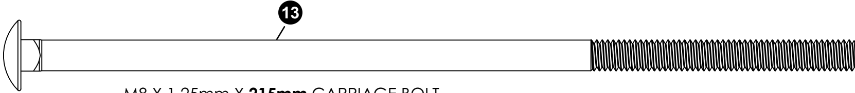
M8 X 1.25mm X 215mm CARRIAGE BOLT for poles 4"-6" 1B-7259-00 QTY. 4
