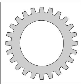
While performing step 9 in the owners manual add the serrated lock washer in between the lamp base and the pole section "A".
