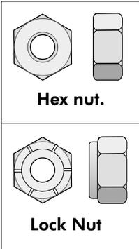
Remove hex nuts shown, on both light assemblies, and replace with lock nuts. **Note: If necessary, use a standard screwdriver to keep nut from spinning while tightening.**
