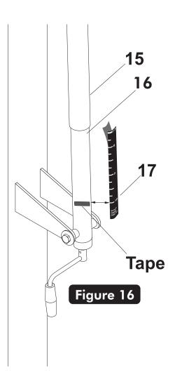
25. Remove the adhesive backing from the Height Decal (#17). Next, carefully align and stick decal to backside of steel actuator (#16) starting at the 10 ft mark first. Be sure to keep the height decal straight and rub out all air bubbles. See Figure 16.
