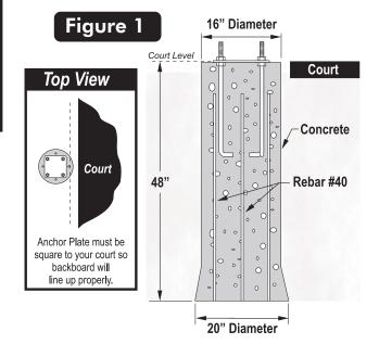
Note: Using a concrete form for the top 4" of the concrete is recommended. Cardboard forms can be purchased at some hardware and home stores or a wooden form can be constructed out of  $2 \times 4$ 's.
