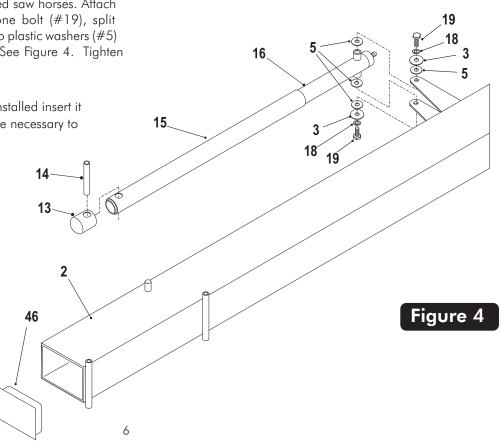
NOTE: It is important for the installer to understand the necessity of the Plastic washers (#5) provided. These washers adequately space painted parts at all pivot points. Neglecting the use of these washers will result in rusted parts.
