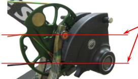
Press must ONLY apply pressure to the limbs in this area.
